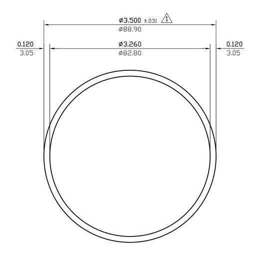
0.120(3.05)WALL THICKNESS EXCEPT AS SHOWN DATE REV DESCRIPTION BY 03/10/23 NDZAL REMOVED EXPOSED SURFACES AND ALLOY 07/15/15 1 ADDED ±.031 TOLERANCE. PAUL IN.<sup>2</sup> 822.089 мм.2 1.274 EST.AREA EST.AREA 2.276 EST.WT. 1.529 LBS/FT. EST.WT. KG/M. 21.237 539.424 EST.PER. MM. EST.PER. 10.996 279.3 OUT PER. MM. OUT PER. 3.500 C.C.D. 88.900 C.C.D. FACTOR 14 FINISH M/F ALLOY & TEMP.
